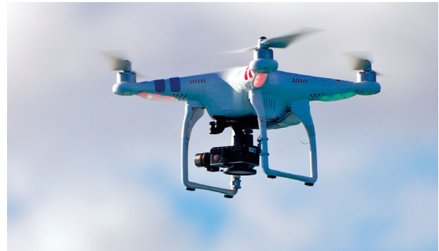
Fig. 2. DJI Phantom II® unmanned aerial vehicle (UAV) quadcopter equipped with a video camera GoPro Hero 3+ Silver edition used for this study (photo credit: Valere Sabatier)
